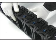
Assembly the Skid on the entire connected Side
