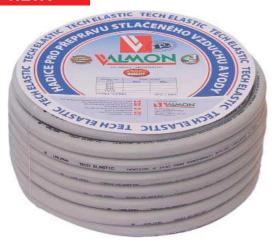
Very elastic PVC hose for the transport of pressurised air and water, specially designed for the distribution of pressurised air, for connection of pneumatic tools, spray pistols, sprayers, etc. The excellent elasticity of the hose is also ensured at very low ambient temperatures (down to -20°C). These hoses are certified for drinking water transport.
