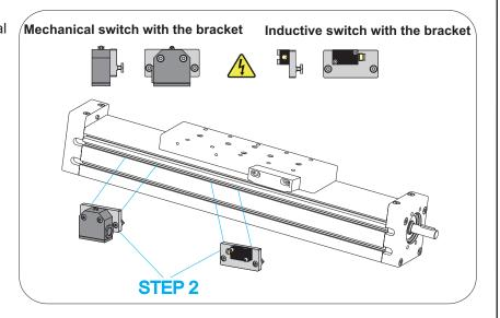
**STEP 3:** After the mechanical or inductive switch with bracket is placed in the desired place in slots, tighten the screws of the bracket.
