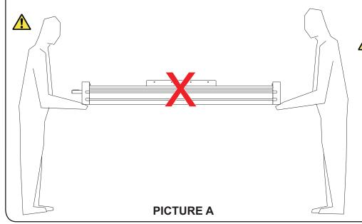
Carrying the Linear Unit holding the END BLOCKS isn't allowed, it must be carried holding the PROFILE of the Linear Unit.
