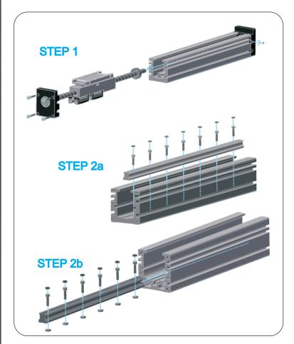
**Note:** when replacing the rail consider that if the rail is damaged it is possible that the carriage is also damaged. We recommend that you change rail and carriage together as this is the only way to ensure smooth operation.
