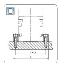
The modules are mounted by using fixtures which are placed in the slot on the side of the profile.
