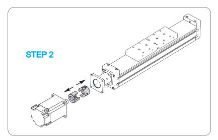
**STEP 2**: Place the coupling halves on the drive journal of the Linear Unit and the motor.
