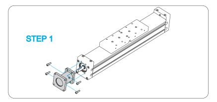
**STEP 1:** Attach the motor adapter on a preprepared location on the Linear Unit and screw down.
