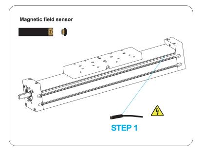
**STEP 1:** The magnetic field sensor must be placed in the slot of the profile, that is made for this purpose.
