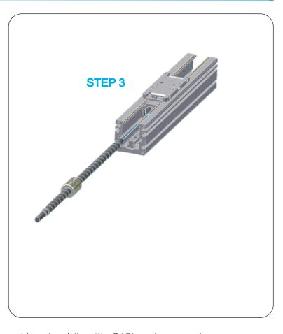
**Note:** all the screws (except set screws) must be glued (Loctite 243) and screwed with the torque specified in the table on page 1.005.0 unless written otherwise at the individual steps.
