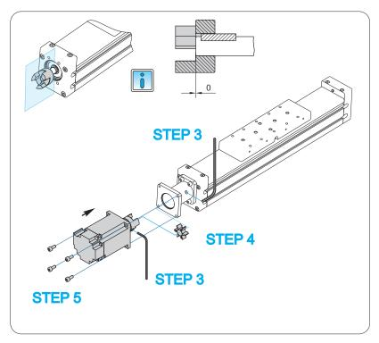
**STEP 3:** Ensure that the coupling halves and the drive journals are correctly aligned.
