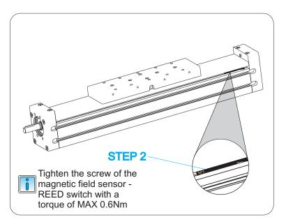
**STEP 2:** After the magnetic field sensor is inserted and positioned in the right location in the slot, tighten the screw of the sensor.
