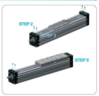
Note: all the screws (except set screws) must be glued (Loctite 243) and screwed with the torque specified in the table on page 1.005.0 unless written otherwise at the individual steps.
