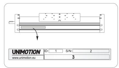
The label must be fully visible (in particular details of the serial number) and must ensure compliance with all the instructions contained on it. Damaged or illegible labels must be replaced.
