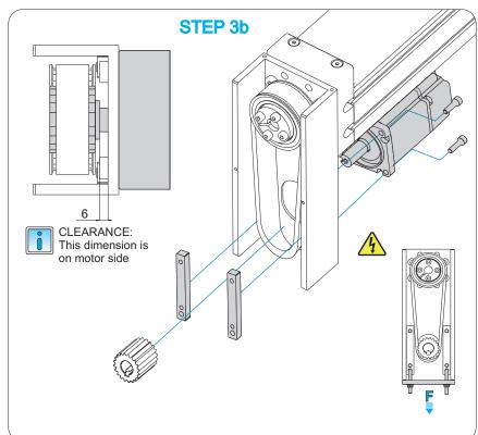
**STEP 3b:** Mount the motor onto the housing and tension lightly the tightening screws of the motor. When the motor is mounted, mount the belt sprocke tension unit onto the motor journal.
