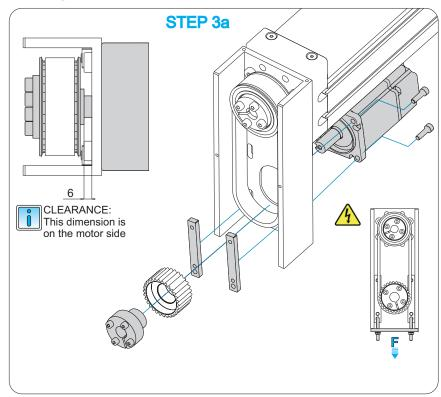
STEP 3a: Mount the motor onto the housing and lightly tension the tightening screws of the motor. When the motor is mounted, mount the belt sprocket with the tension unit onto the motor journal. Adjust the clearance as shown in the picture. Tension the tension unit. Tension the motor with the belt with the pretensioning force F and tighten the motor down on the housing. The pretensioning force F depends of the size of the Linear Unit and motor.
